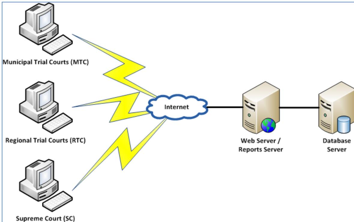
Figure 3.3: Hardware and Network Configuration
